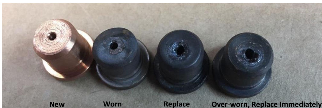
Figure 14: Levels of nozzle wear.
